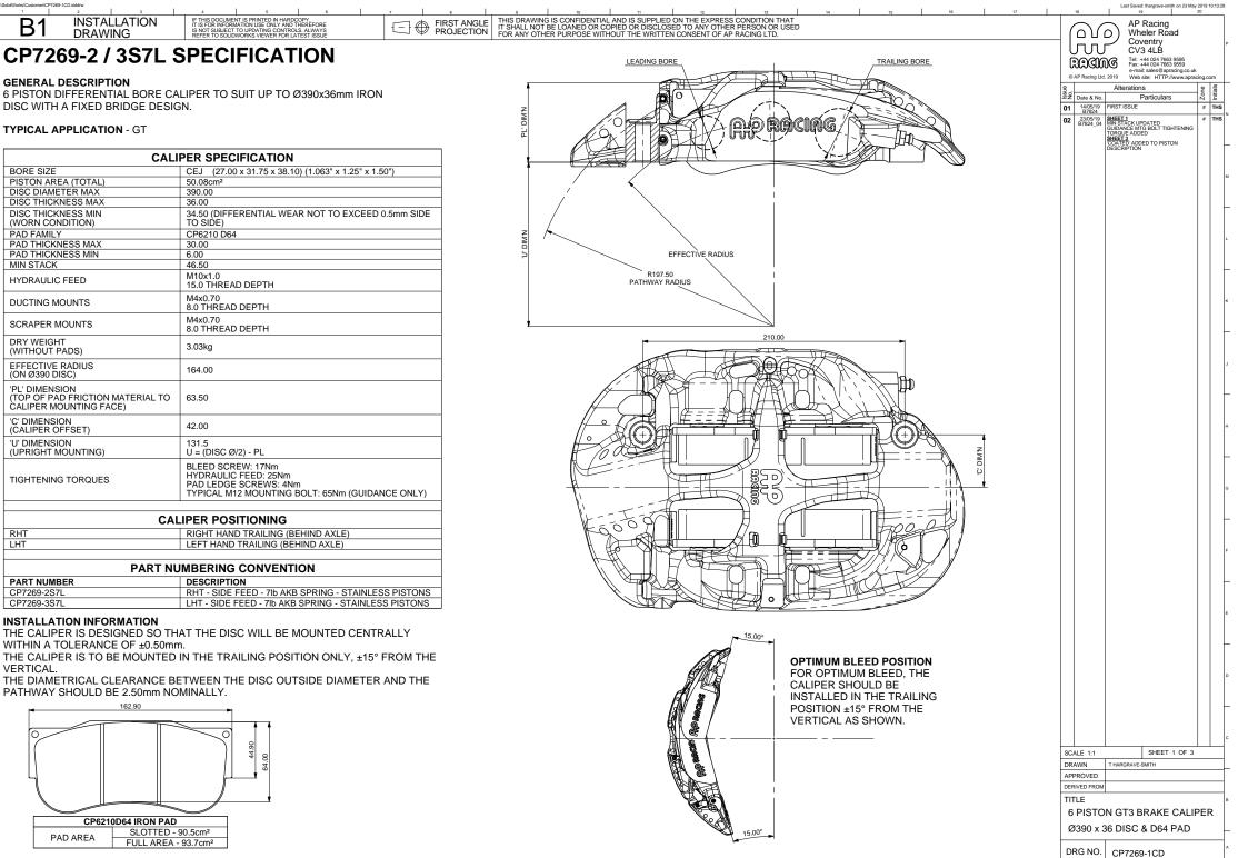
DISC THICKNESS MIN (WORN CONDITION) PAD FAMILY PAD THICKNESS MAX PAD THICKNESS MIN MIN STACK HYDRAULIC FEED DUCTING MOUNTS SCRAPER MOUNTS DRY WEIGHT (WITHOUT PADS) EFFECTIVE RADIUS (ON Ø390 DISC) 'PL' DIMENSION (TOP OF PAD FRICTION MATERIAL TO CALIPER MOUNTING FACE) 'C' DIMENSION (CALIPER OFFSET) 'U' DIMENSION (UPRIGHT MOUNTING) TIGHTENING TORQUES
